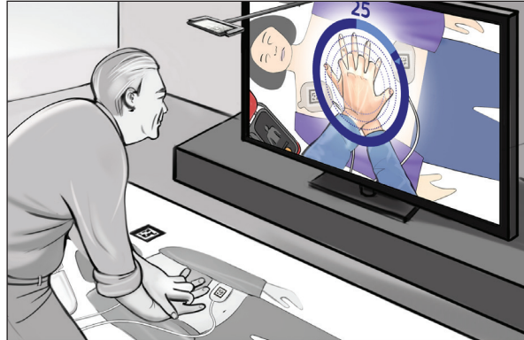
An auditory beat and visual feedforward indicate 110 compressions/min. with optimal depth and release. A timer shows how much longer he needs to continue. Trying to keep pace, John realises how physically demanding resuscitation is.
