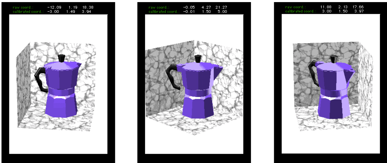
Figure 4, Three perspectives according to the Delft Virtual Window System projection method generated by three different head positions. From left to right: viewed from the left, from the middle and from the right.
