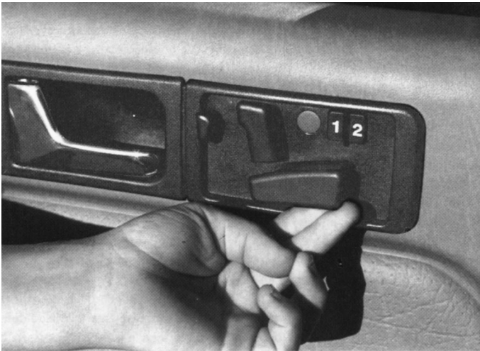
Figure 3.9 Control for car seat adjustment in a Mercedes (Norman, 1988).
