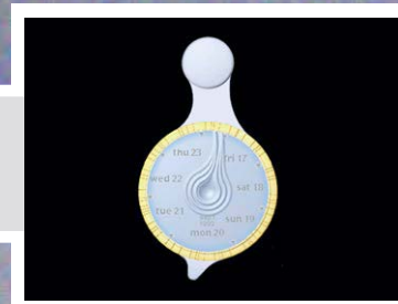
Turning the rotary dial of this PDA causes an elegant circular flow of characters over the screen.
