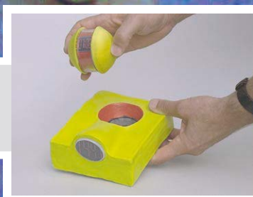
The further the ball is placed from the base unit, the more insistent the alarm clock will be in the morning. Fetching and placing the ball over the speaker muffles the sound (design: O.J. De Groot and M. Van de Velden).
