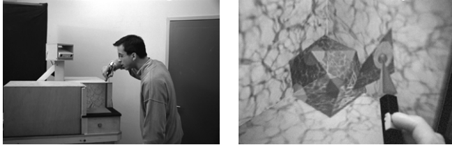
Figure 6 In Cubby the user can manipulate virtual objects at the place where they appear by means of an augmented instrument.
