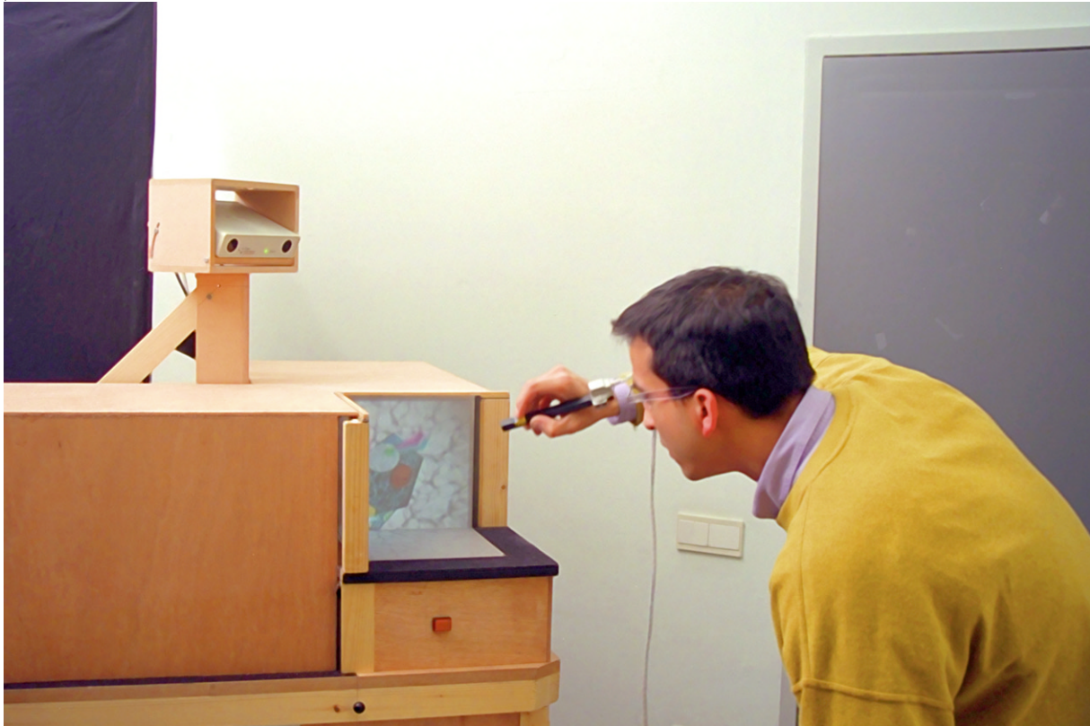
Figure 1 Cubby is a unified VR system: the user manipulates virtual objects at the place where they appear.
