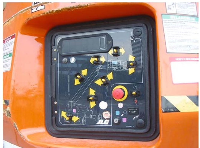
Fig. 4 A graphical variant of natural mapping: the controls are placed in a perspective line drawing of the crane itself
