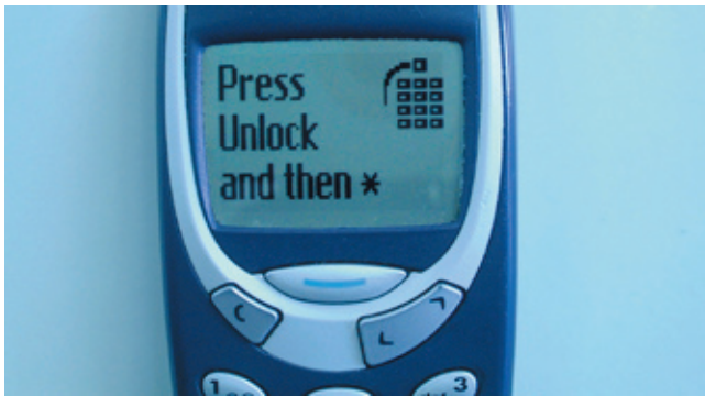
Figure 1: Augmented Feedforward. The display of mobile phone informs the user about the appropriate action that needs to be taken to unlock the keypad.
