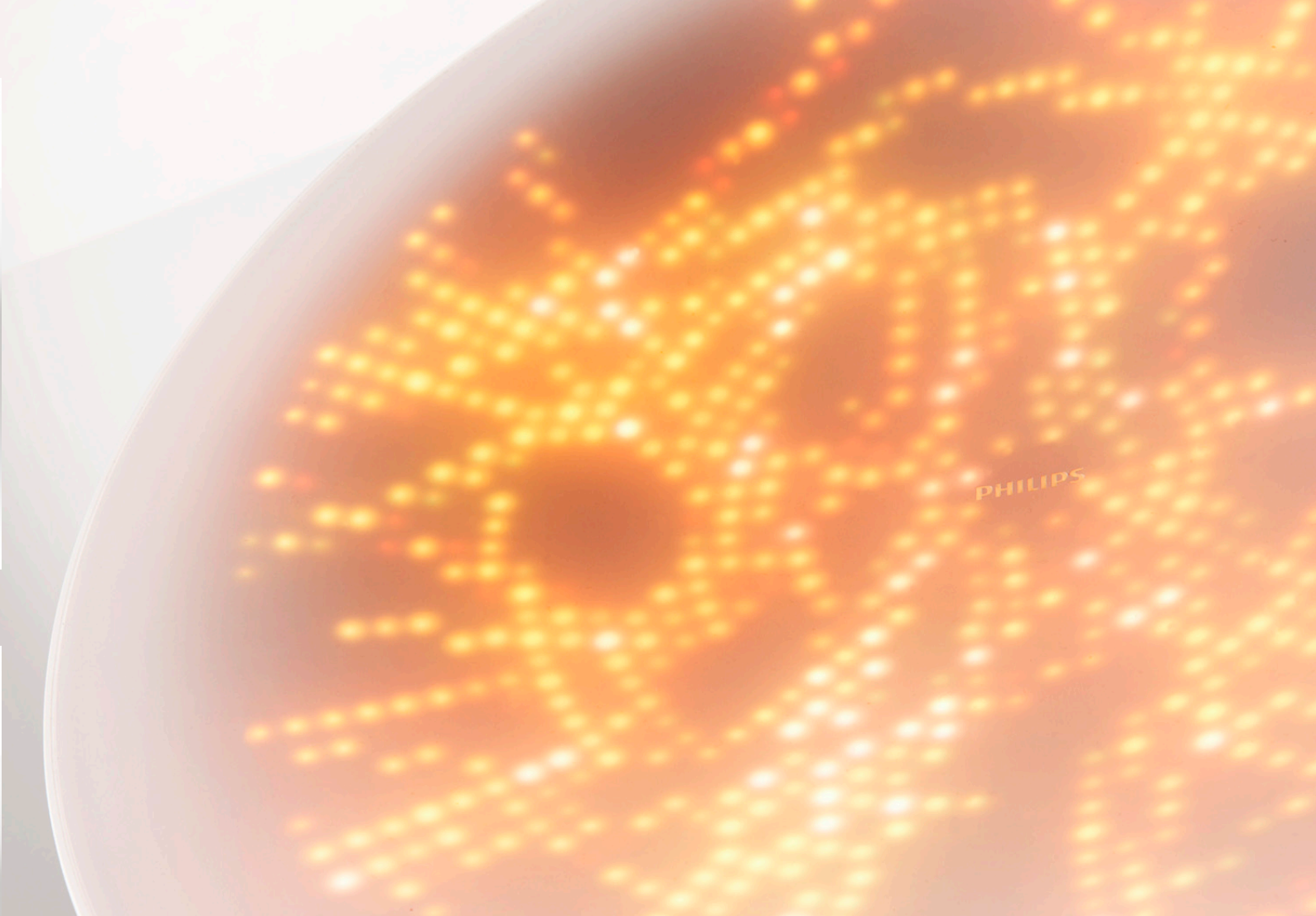
Figure 12. The EmoBowl can function as a 'high-res luminaire': the 1600 LEDs together are the equivalent of a 100W light bulb
