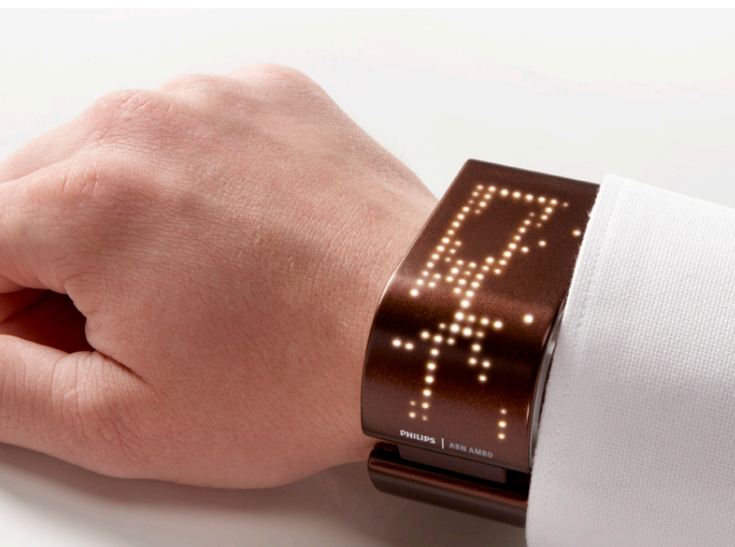
Figure 7. EmoBracelet in alert mode, corresponding to high-arousal.
